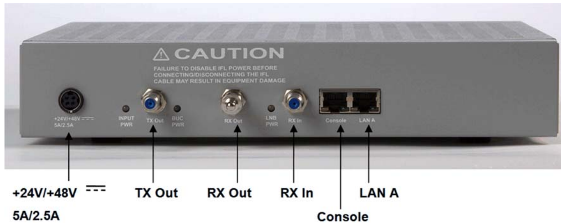
Figure 10 iDirect 3000 series™ Satellite Router Rear Interface Connectors
