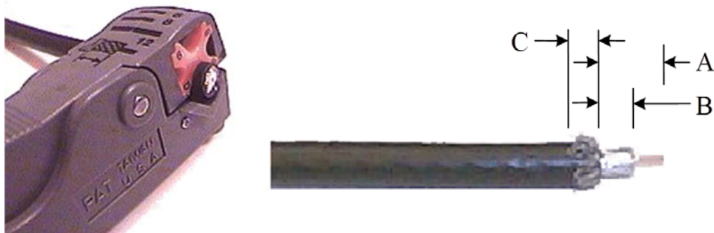
Figure 13 Cutting Technique for Removing Foil in the Braid
