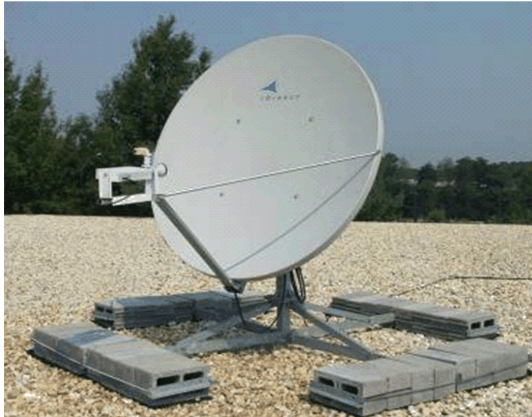
Figure 7 Typical Antenna with BUC and LNB
